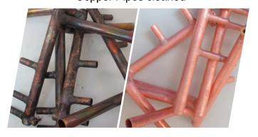
Thermal deburring removed
