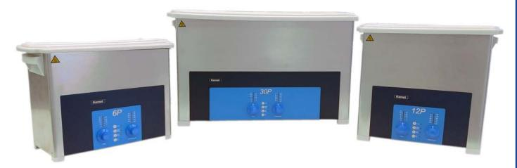
Top of the range digital generator operates piezo-ceramic transducer elements giving a powerful cleaning effect. The Booster function, for extra power, can be used for the most difficult cleaning tasks. Distribution of the ultrasonic energy is achieved by the frequency sweep to give precision cleaning throughout the tank. All models are equipped with thermostatically controlled heating to ensure optimum cleaning temperature.
