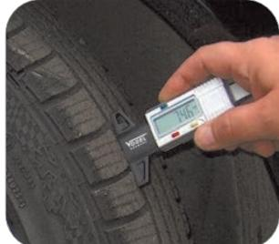
round probe tip ( $\varnothing$  1.5 mm)
