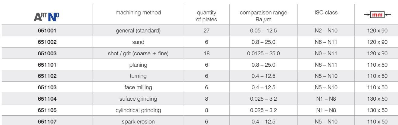
The image shows the RUGOTEST 1 specimen plate dimensions table, which lists the number of plates, comparison range, ISO class, and size for various machining methods.
