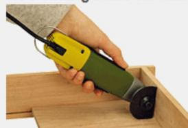
Oscillates, making it ideal for cutting metal, wood, PC cards, plastics, plaster of Paris and many other materials. The segment cut facilitates exact cutting right into corners.
